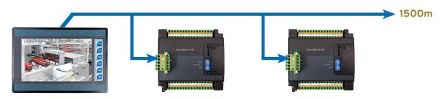
CsCAN supports up to 253 nodes with a maximum network distance of 1500 meters.
