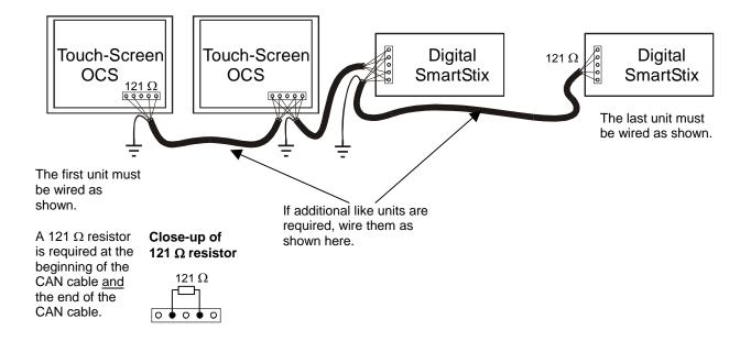
Figure 13 - CAN Wiring between Touch Screen OCS and Digital SmartStix Modules
