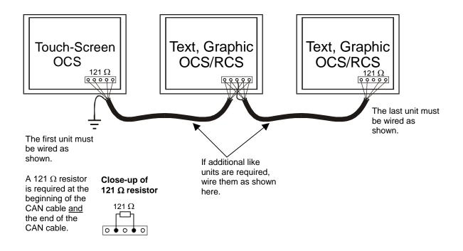
Figure 15 - CAN Wiring between Text, GraphicOCS, RCS and Touch Screen OCS
