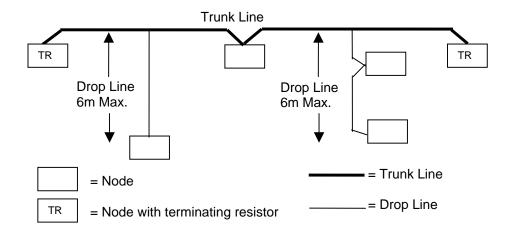
Figure 17 – Trunk/Drop Line Topology
