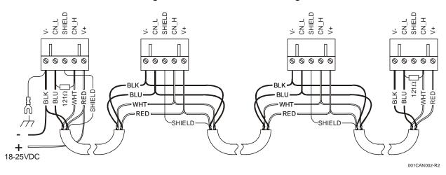
Figure 5 – CAN Wiring Drawing
