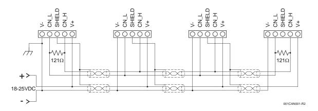
Figure 4 – CAN Schematic Drawing
