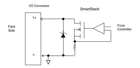
Specification for transient voltage suppressors (transorbs) used on output circuitry is 43 V, 1500 W.
