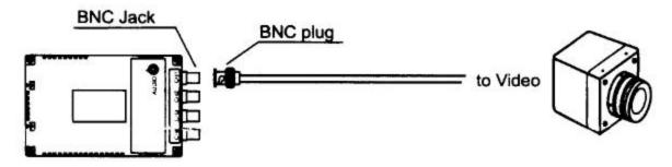
Figure 5 – BNC Jack and BNC Plug
