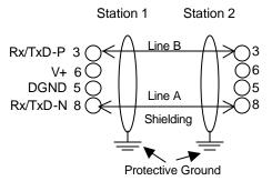
**b.** It is necessary to terminate both ends of the network. Both terminations must have power to them to insure proper operation of the network. The following diagram illustrates the correct connection for the termination resistors. The diagram is for illustrative purposes only.
