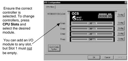
Figure 3.1 – Select the Module Slot
