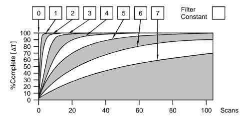
**Digital Filtering**. The illustration above demonstrates the effect of digital filtering (set with Fillter Constant) on module response to a temperature change.
