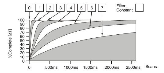
**Digital Filtering**. The illustration above demonstrates the effect of digital filtering (set with Filter Constant) on module response to a temperature change.
