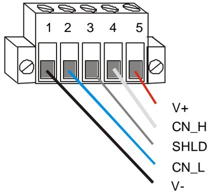
Figure 2.1 – Network Connector for the CDC200 (CAN Port)
