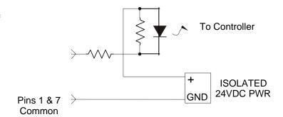
This circuit is typical of **Encoder A, Encoder B, and Marker** *inputs.*
