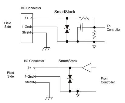
Specification for transient voltage suppressors (transorbs) used on output circuitry is 11 VDC, bidirectional 500 W.
