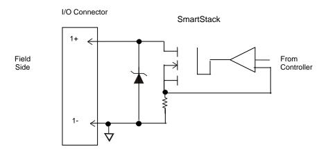
Specification for transient voltage suppressors (transorbs) used on output circuitry is 43V, 1500W.
