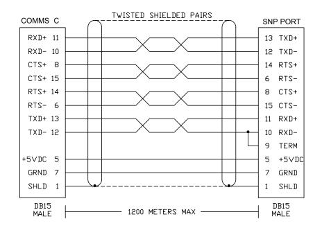
**Note**: The standard SNP cable includes the wire from pin 5 to pin 5. This wire is not neccessary if you are building a custom cable.
