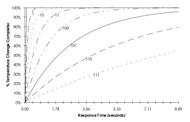
**Digital Filtering**. The effect of digital filtering (set with Byte 2) on module response to a temperature change. (% temp change completed vs. time).
