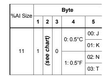
**Configuration Parameters**. Byte 2 sets digital filtering, Byte 4 sets the module resolution, and Byte 5 sets the thermocouple type.
