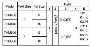
**Configuration Parameters**. Byte 2 sets digital filtering, Byte 3 sets the module resolution, and Byte 5 sets the thermocouple type.
