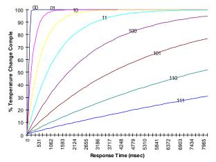
**Digital Filtering**. The effect of digital filtering (set with Byte 2) on module response to a temperature change. (% temp change completed vs. time).
