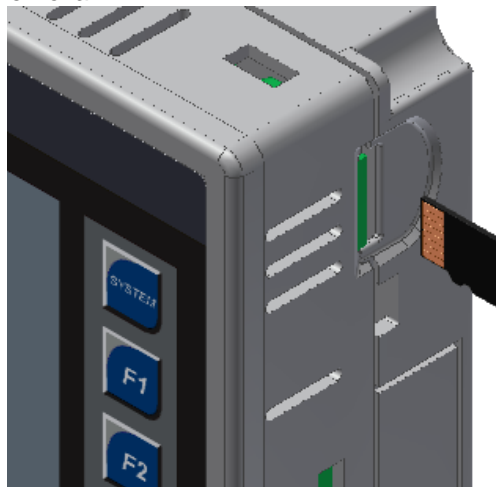
Figure 9.2 – Installing Removable Memory Card
