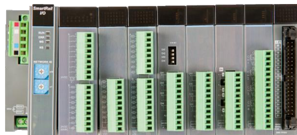
HE599COS100, with 8 I/O modules installed.
