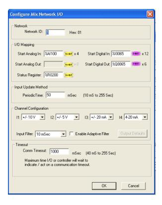
**Network ID** - This should match the ID of the rotary switch on the SmartBlock unit and should be unique to the network.
