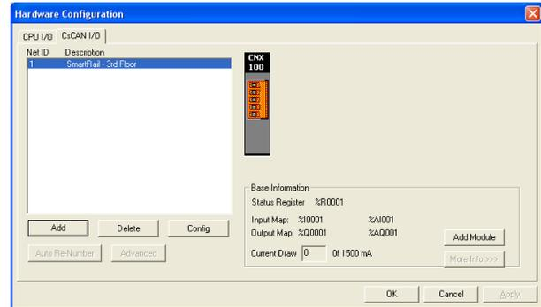
8. Now up to 8 modules can be added via the “Add Module” button. As I/O modules are added the Input Map, Output Map, and Current Draw are updated, showing the accumulated I/O Module Information. More details regarding each module can be viewed via the “More Info” button.
