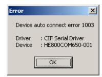
When downloading for the first time or if HSyCon is not able to auto-connect it will be necessary to select a COM port. The window shown below will pop up when an online function is started and the desired COM port should be selected. HSyCon supports COM 1 through COM 4.
