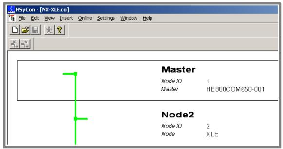
The Global State Field allows scrutiny of the Master and all of the slave nodes on the network. The connection status of each individual slave can be quickly checked from the Device Specific Status Bits window. Below is an example of the XLe connected and active at node 2 indicated by the 2 highlighted in green.
