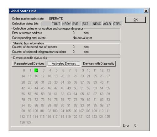
Errors that occur will result in one of the status bits (TOUT, NRDY, EVE, FAT, NEXC, ACLR, or CTRL) being highlighted. The definitions of these status bits can be found in the HSyCon help file. For more specific information on faults for individual slaves click on '**Devices with Diagnostic'**. The nodes with errors will be highlighted in red. For more information on the error double click on the specific node number in question.
