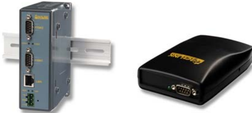
Figure 1 – Connect a serial-to-Ethernet gateway, such as ABLELink’s GW21R Dual Port Industrial Serial Server or GW21E Single Port Serial Server, to the LX serial port.
