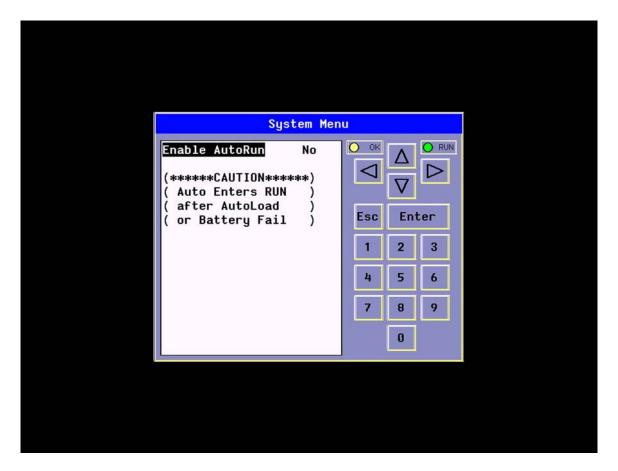
Figure 14.12 – Enable AutoRun Yes/No System Menu
