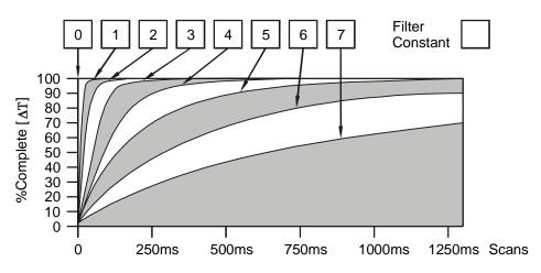
*Digital Filtering*. The illustration above demonstrates the effect of digital filtering (set with Filter Constant) on module response to a temperature change.
