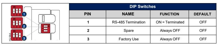
The DIP switches are used to provide a built-in termination to the MJ2 port if needed. The termination for these ports should only be used if this device is located at either end of the multidrop/daisy-chained RS-485 network.
