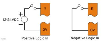
Digital inputs may be wired in either a Positive Logic or Negative Logic fashion as shown. The setting in the Cscape Hardware Configuration for the Digital Inputs must match the wiring used in order for the correct input states to be registered. No jumper settings are required for XLEe/XLTe. When used as a normal input and not for high speed functions, the state of the input is reflected in registers %I1 – %I12.
