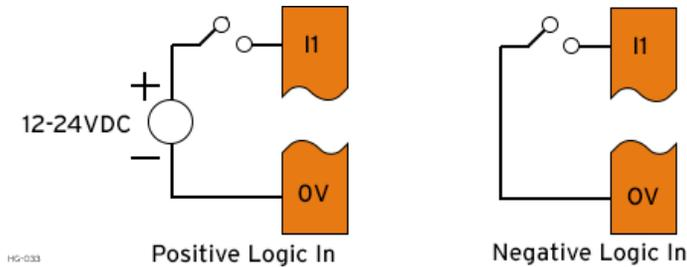
Digital inputs may be wired in either a Positive Logic or Negative Logic fashion as shown. The setting in the Cscape Hardware Configuration for the Digital Inputs must match the wiring used in order for the correct input states to be registered. No jumper settings are required for XLEe/XLTe. When used as a normal input and not for high speed functions, the state of the input is reflected in registers %I1 – %I12.
