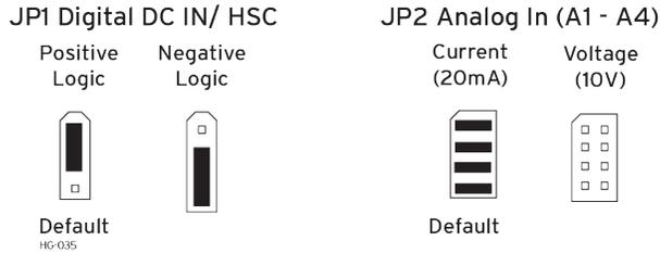
**NOTE:** The Cscape Module Configuration must match the selected I/O (JP) jumper settings.
