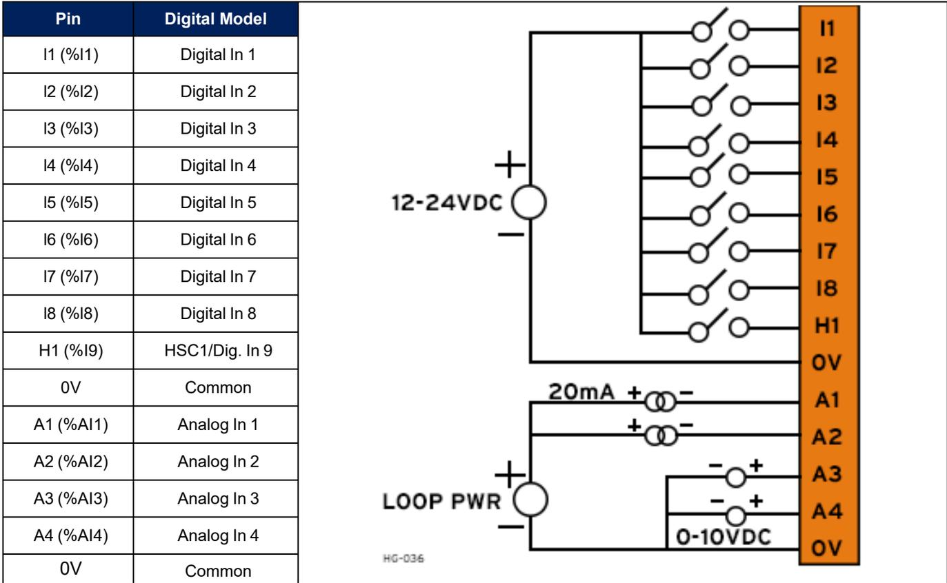
**NOTE:** The 0V terminals are internally connected.
