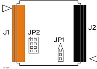
Location of I/O jumpers (JP1 & JP2) and wiring connectors (J1 & J2) with back cover removed.
