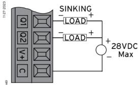
Sinking: Outputs can sink 500mA
