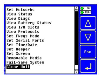
Step 2: Selecting "Clone Unit" menu will open the following menu screen. Select "Load Clone".
