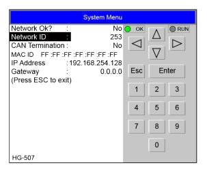
This submenu allows setting for the CAN and Ethernet network to be viewed or changed.
