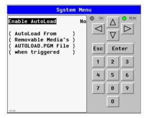
Enable AutoLoad No = Does not load AUTOLOAD.PGM automatically when application program is absent or corrupted.
