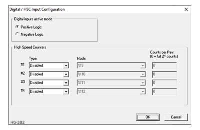
The Active mode group box allows the user to select if inputs are active high (Positive logic) or active low (Negative logic). It is important that this setting matches the jumper settings on the hardware.
