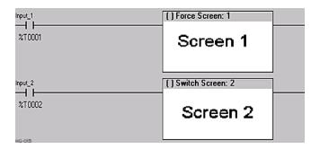
There is also a system register that can be used to for control-based screen navigation. %SR1 can be read to determine the current screen or written to change the current screen.
