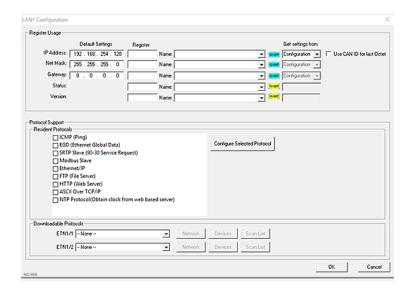
If **Get settings from** is set to **Configuration** for any parameter, the addresses in the **Default Settings** column will take place when this program is loaded and every time this controller enters RUN mode. Registers may optionally be defined that will reflect the settings. These settings may temporarily be changed via the SYSTEM menu but will revert to the Cscape-configured settings at any transition into RUN mode, i.e. a program download or at power-up.
