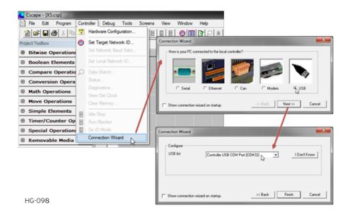
If **Controller USB COM Port** is not present in the dropdown list, the Windows operating system has not yet recognized the OCS as an installed device. Be sure the installation process is complete and that the correct drivers are installed. The Connection Wizard must be completely closed and reopened to refresh the USB dropdown list.
