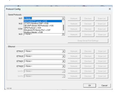
**NOTE:** If the MJ1 port is to be used in the Protocol Config, it will no longer be available for Cscape programming unless the controller is put into IDLE mode.
