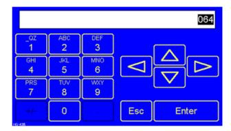
Once the desired value is entered, pressing the **Enter** key moves that value into the object (and the corresponding OCS register) and the alpha-numeric keypad disappears. Alternately, pressing the bkey any time before the **Enter** key cancels the operation, leaves the objects current value unchanged, and the alpha-numeric keypad disappears.
