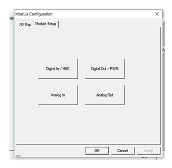
The Module Setup allows a user to configure four types of I/O. **NOTE**: Not all controllers offer all four types. Refer to the controller's datasheet on the Horner website's <a href="Documentation Page">Documentation Page</a> for more information regarding specific models.
