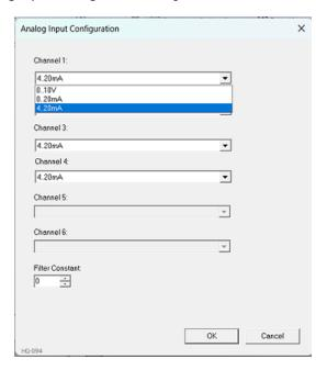
The Channel x drop down windows allow the user to specify the mode for each analog input to operate. The Channel x drop down windows are enabled/disabled according to which model is being configured. All of the models have the following modes available:
