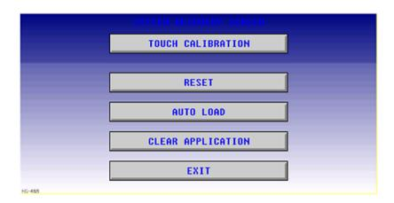
**NOTE**: Advanced options, accessed by holding the system key down, may be locked out from user access. If holding the SYSTEM key does NOT respond, verify that the system menu's Set Fkeys submenu's parameter SYS\_Fn is enabled.
