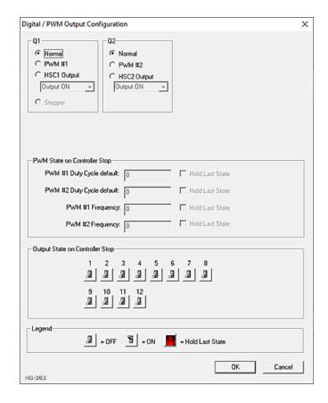
The Q1 and Q2 group boxes allow the user to specify the operation of the multifunction outputs.
