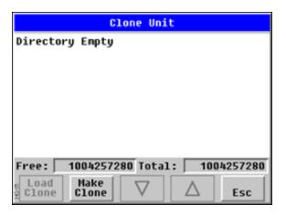
**Load Clone** and **Make Clone** virtual buttons are below the screen. **Free/Total**: Displays number of Free and Total bytes in Removable Media.
