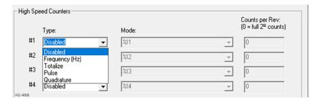
The mode drop-down items are set according to the type selection. The Counts Per Rev. window is enabled/disabled according to the type selection as well.
