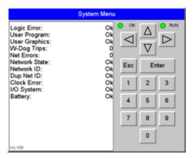
The View Diags submenu displays up to 11 System Diagnostics, none of which are editable. The first two System Diagnostics are critical. If any of them indicate a Fault condition, the X7 OCS will not enter or remain in Run mode, and the problem must be investigated and corrected.
