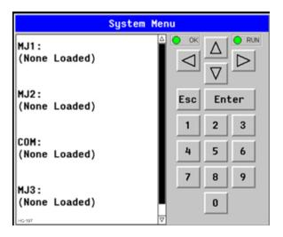
The View Protocols submenu displays currently configured serial protocols. The configuration is not editable from the System Menu.
