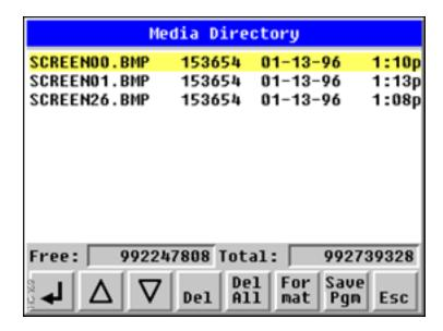
The currently selected entry is indicated by a yellow highlight which can be moved up or down by touching the arrow buttons or by directly touching an entry. If more entries exist than can fit on the page, a scroll bar is displayed on the right side that also indicates the current relative position.
