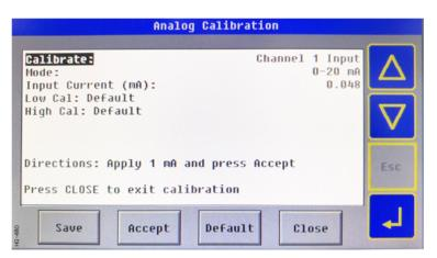
The "Calibrate:" options allows selecting the individual input and output channels. Start by pressing select and using the up and down arrows to select the appropriate channel to calibrate. Next, the mode for the analog (if applicable) is selected using the "Mode:" option.
