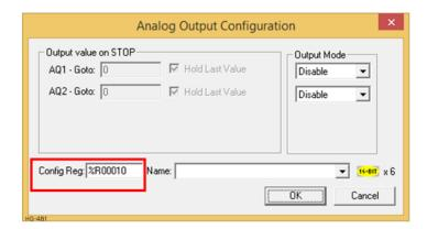
The **Output value on Stop** group box contains items that allow the user to specify how the analog output channels behave when the controller is stopped. The outputs can either hold their value or default to a value when the controller is stopped.
