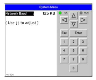
The Set Network Baud submenu for both X7 models displays just one System Setting and it is editable.
