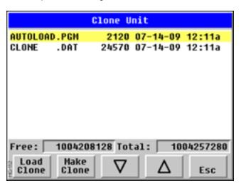
**Step 3**: User needs to confirm Load Clone as shown below:
