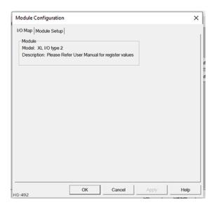
The Module Setup allows a user to configure four types of I/O. **NOTE**: Not all controllers offer all four types. Refer to the controller's datasheet the using Horner's <u>Documentation Search</u> page.
