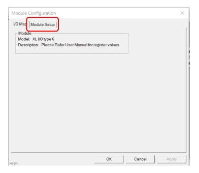
The Module Setup allows a user to configure four types of I/O. **NOTE**: Not all controllers offer all four types. Refer to the controller's datasheet on the using Horner's <u>Documentation Search</u> page.
