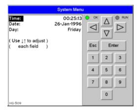
The Set Time/Date submenu displays three System Settings. Time and Date are editable, and Day is automatically calculated from the Date setting.
