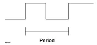
At controller power-up or during a download, the PWM output is maintained at zero until both the Frequency and the Duty cycle are loaded with non-zero values.
