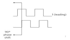
Using the above waveforms and a HSC input configuration of "Quadrature" - "1 leads 2, count up," the accumulator will count up when 1 is rising and 2 is low, 1 is high and 2 is rising, 1 is falling and 2 is high, and when 1 is low and 2 is falling. This results in 4 counts per revolution. So in order to determine the number of cycles, the accumulator would have to be divided by 4.
