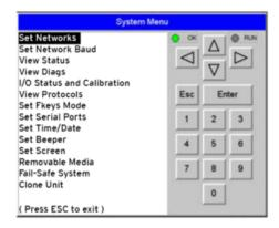
As mentioned above, the System Menu is started by pressing the System key on the X7 OCS. Next press ESC to exit the System Menu, or use ↑ and ↓ to select an item and press the **Enter** key to display the item's submenu.
