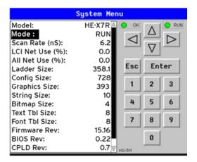
The View Status submenu displays up to 18 System Settings. Only the Mode System Setting is editable.
