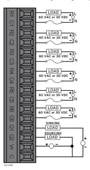
**Protection for Inductive Loads** – Inductive loads can cause reverse currents when they turn off that can shorten the life of relay contacts. Some protective measures must be determined by an engineer. Below are some recommendations that will work for many applications. If there are additional questions on protection from inductive load, consult Horner Technical Support.
