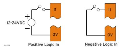
In positive logic mode a positive voltage applied to the input will turn the input. The internal design of this mode is basically a resistor from the input to I/O ground. This mode is sometimes called sourcing.
