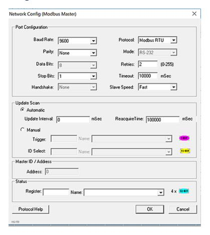
Network Configuration provides the required parameters to configure the network. Each protocol is different and may not require the entire Network Config field. Please refer to the table below for the options in the Network Config field.
