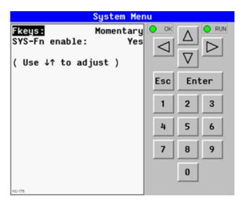
The Set Fkeys submenu displays two System Settings, both of which are editable.
