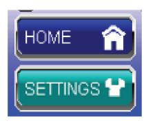
Screen jumps can also be triggered on other keys or based on control logic for more advanced applications. To allow the operator to change screens, a **screen jump object** is generally used. This object may be visually **represented as a button** (responding to touch) or remain invisible and logically tied to an OCS register. An optional system ICON may be configured for display along with the legend, which aids in identifying the object as one that causes a screen change.
