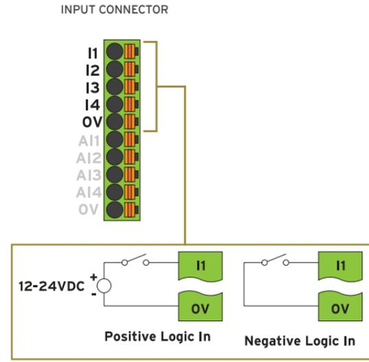
**POSITIVE LOGIC vs. NEGATIVE LOGIC WIRING:**
