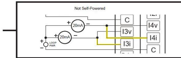
C terminals are connected together internally but isolated from bus and power circuits.
