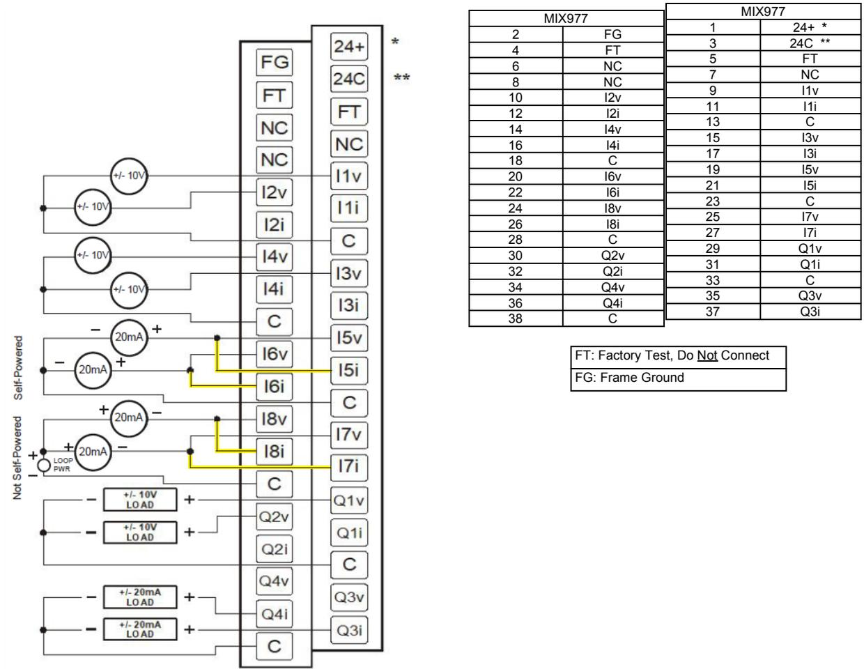
C terminals are connected together internally but isolated from bus and power circuits.
