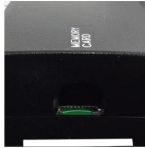
Figure 13.1 - Removable microSD Memory Card Slot
