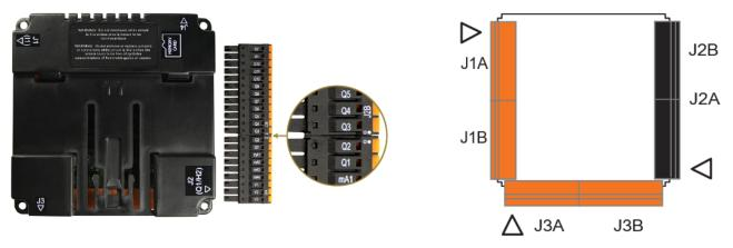
For ease of operability, the high density terminals are divided into more manageable pairs of connectors (J1A + J1B, J2A + J2B, J3A + J3B). To ensure proper installation, connector symbols must match.
