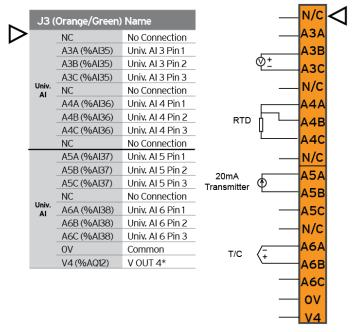
**NOTE**: \* Both mA & V outputs are active for each output channel, however, only the configured output type is calibrated (maximum 4 channels simultaneously).
