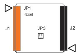
Location of I/O jumpers (JP1 & JP3) and wiring connectors (J1, J2, J3 & J4) with back cover removed.
