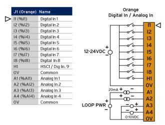
NOTE: The 0V terminals are internally connected.
