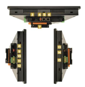
**NOTE:** Use caution when connecting controllers to PCs via serial or USB. PCs, especially laptops may use "floating power supplies" that are ungrounded. This could cause a damaging voltage potential between the laptop and controller. Ensure the controller and laptop are grounded for maximum protection. Consider using a USB isolator due to voltage potential differences as a preventative measure.
