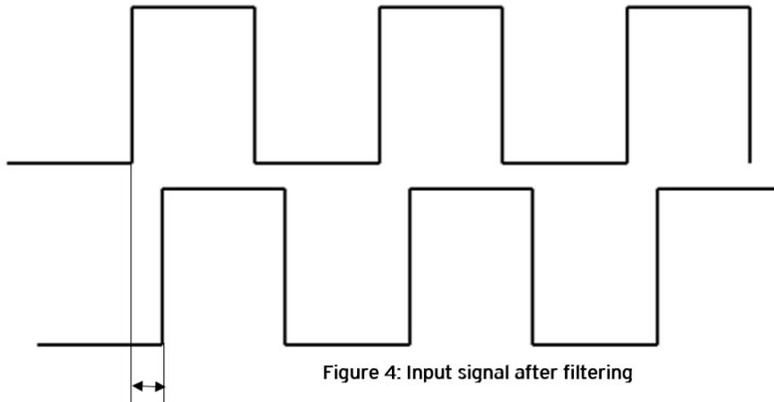
Figure 4: Input signal after filtering
