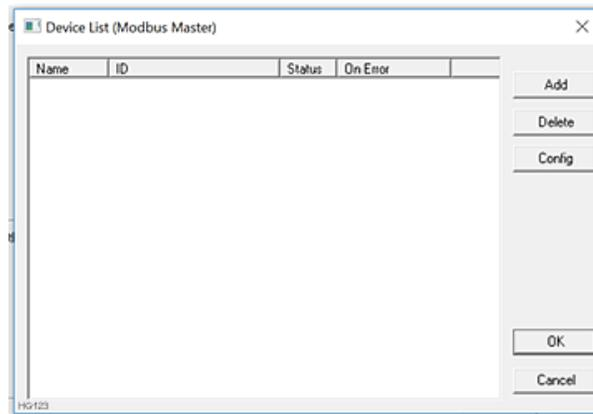
This configuration list is reached from the Device button on the Protocol Config screen and provides a list of the configured devices on the Network. Devices must be created and exist in this list before corresponding Scan List entries can be created for this device. Typically, the number of entries is limited to **64 devices**.
