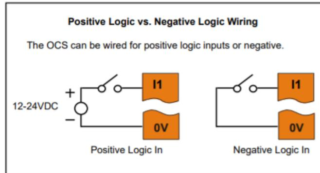
In positive logic mode a positive voltage applied to the input will turn the input. The internal design of this mode is basically a resistor from the input to I/O ground. This mode is sometimes called sourcing.
