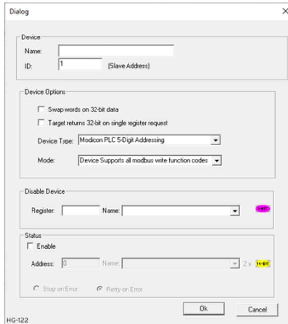
This configuration is reached from the device list when adding or modifying an existing device. While each protocol is somewhat different and can contain protocol specific field, all protocols typically support at least:
