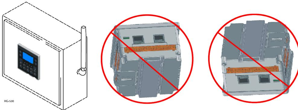
**NOTE—For panel or DIN rail mounting:** The orientation shown above provides for optimum readability of the screen and ease of use of the keypad.
