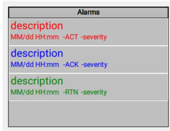
To view, acknowledge and/or clear alarms, the operator must access the alarm viewer. This is accomplished by touching an (enabled) alarm object. When accessed, the alarm viewer is displayed as pop-up alarm viewer dialog.
