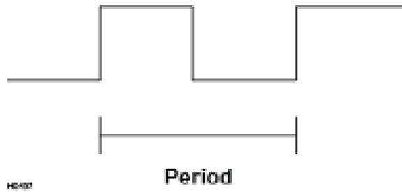
At controller power-up or during a download, the PWM output is maintained at zero until both the Frequency and the Duty cycle are loaded with non-zero values. When the controller is placed in stop mode, the state of the PWM outputs is dependent on the PWM State on Controller Stop configuration. This configuration allows for either hold-last-state or specific frequency and duty cycle counts. Specifying zero for either the period or duty causes the PWM output to remain low during stop mode.
