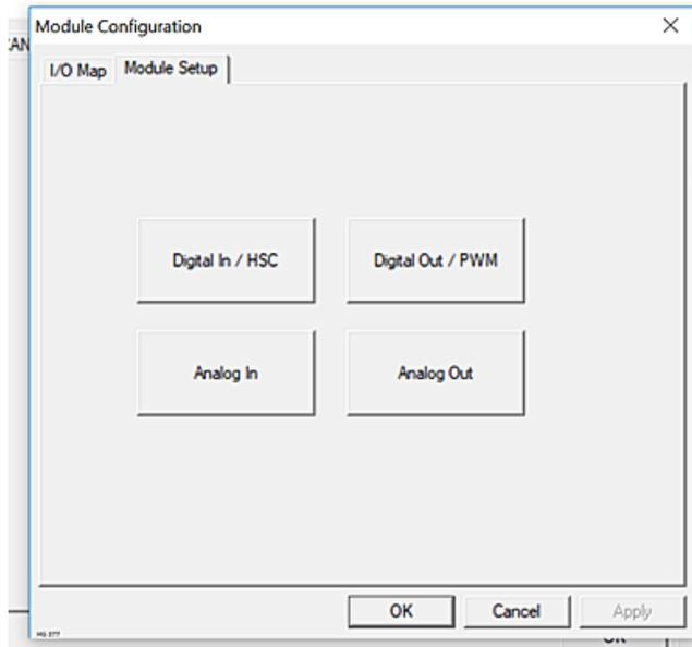
Select **Digital Out/PWM** to open the **Digital / PWM Output Configuration** dialogue.
