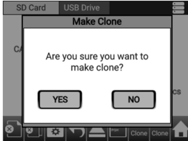
Make/Create clone can also be triggered by setting %SR164.9 bit to “1” from Ladder program or graphics. Once the operation is completed, this bit is made zero by the firmware. When Make Clone operation is triggered by this SR bit, it does not ask the user for confirmation for making clone. The success / failure of the operation is also not notified on screen to the user.
