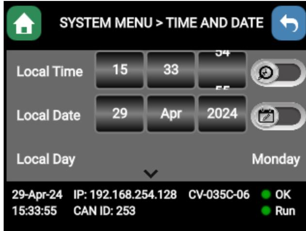
**To Set Time Zone:** The Time Zone setting is an hourly offset from UTC time. If using the Time Zone setting, set it first, then set the local time. UTC time will be automatically set based on the time zone and local time settings.
