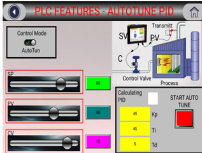
Multiple objects are provided for displaying data such as virtual panel lights, push buttons, numeric value displays, bar graphs, meters, graphs and animated bitmaps. On the Canvas 4, these graphical objects (through ladder manipulation of attribute bits) can change color, flash, or change visibility to attract operator attention.
