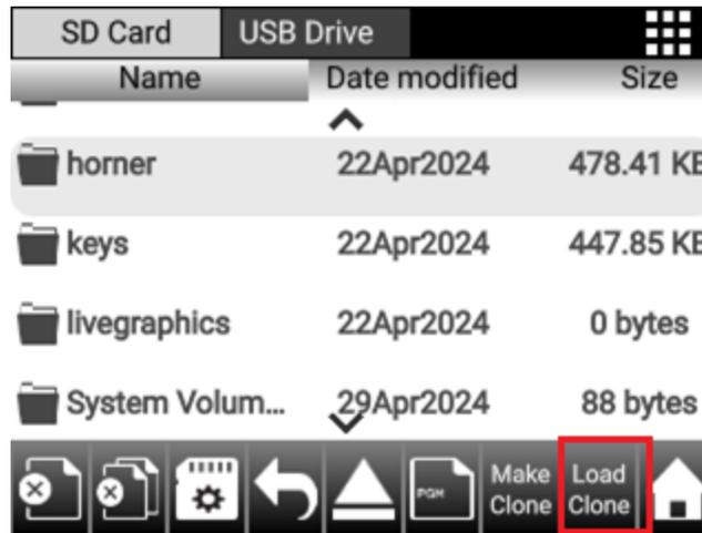
**Step 2:** Select “Load clone” in the menu option at bottom of the screen, “Load Clone” popup window will get open then select Yes to “Load clone”.
