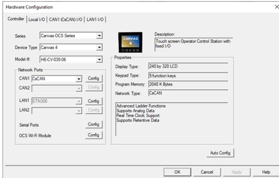
The IP address, Net Mask, and Gateway of the controller may be temporarily set from the System Menu under the Set Networks menu item. Once running or power cycled the configuration will come from the Cscape configuration stored in the unit.
