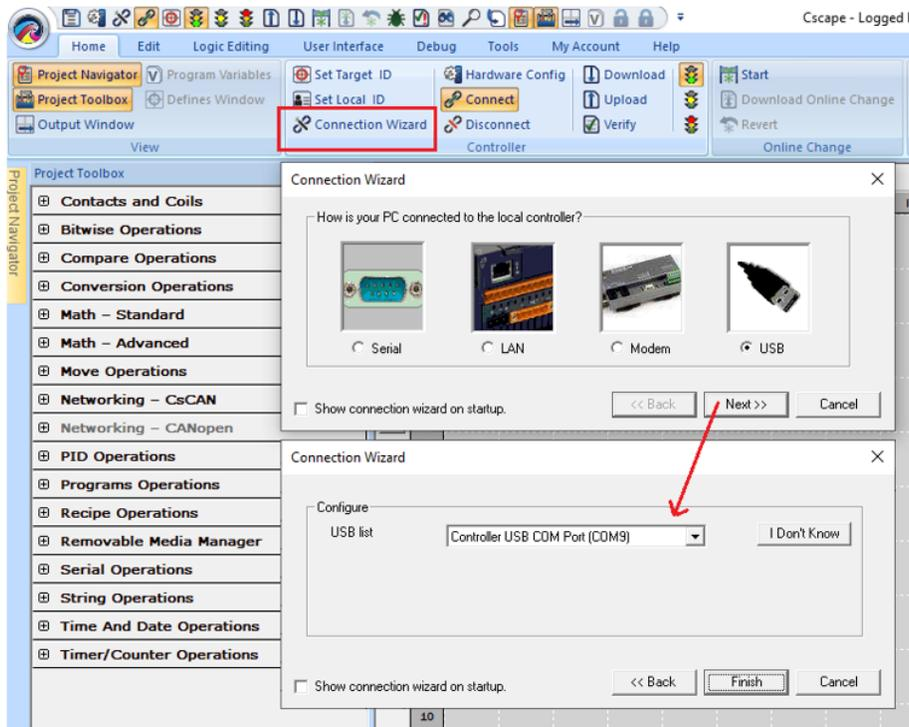
If **Controller USB COM Port** is not present in the dropdown list, the Windows operating system has not yet recognized the OCS as an installed device. Be sure the installation process is complete and that the correct drivers are installed. The Connection Wizard must be completely closed and reopened to refresh the USB dropdown list.
