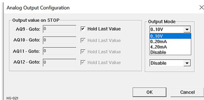
The Output value on Stop group box contains items that allow the user to specify how the analog output channels behave when the controller is stopped. The outputs can either hold their value or default to a value when the controller is stopped.
