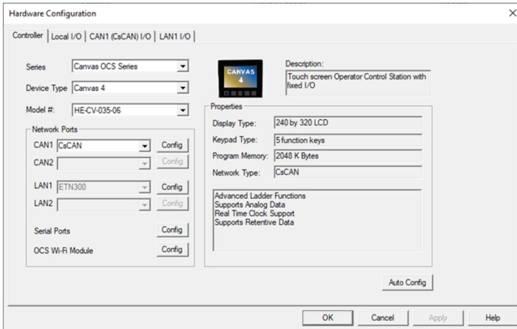
3. Click the **Config** button to the right of the LAN1 for LAN 1 or LAN2 for LAN 2, revealing the Ethernet Module Configuration dialog.
