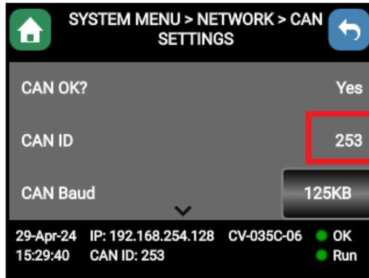
To change the Target ID of Cscape, highlight CAN ID and press **Enter** to provide a new number.
