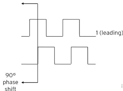
Using the above waveforms and a HSC input configuration of "Quadrature" - "1 leads 2, count up," the accumulator will count up when 1 is rising and 2 is low, 1 is high and 2 is rising, 1 is falling and 2 is high, and when 1 is low and 2 is falling. This results in 4 counts per revolution. So in order to determine the number of cycles, the accumulator would have to be divided by 4.
