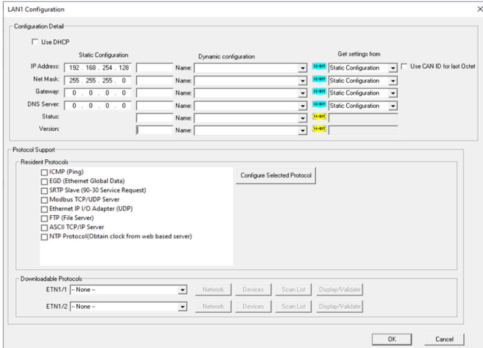
4. Configure the Ethernet Module parameters as follows:
