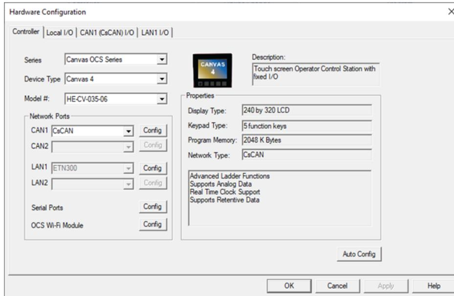
After selecting Local I/O, select the **Config** button next to the I/O connector.
