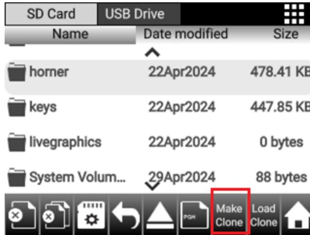
Make/Create Clone option enables user to duplicate/Clone application file, all unit settings and all register values from battery-backed RAM. Selecting Make Clone brings up the screen below for the user:
