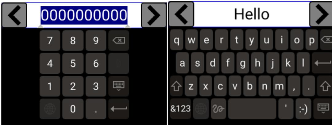
Once the desired value is entered, pressing the Enter key moves that value into the object (and the corresponding OCS register) and the alpha-numeric keypad disappears. Alternately, pressing the ESC key any time before the Enter key cancels the operation, leaves the objects current value unchanged, and the alpha-numeric keypad disappears.
