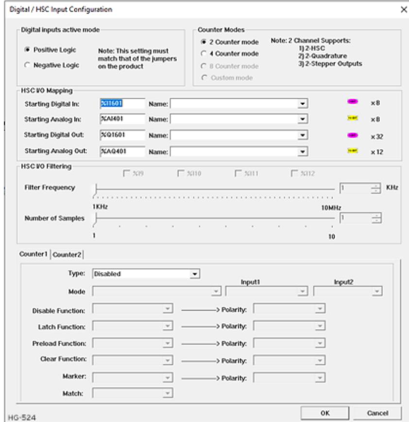
The Active mode group box allows the user to select if inputs are active high (Positive logic) or active low (Negative logic). It is important that this setting matches the jumper settings on the hardware.
