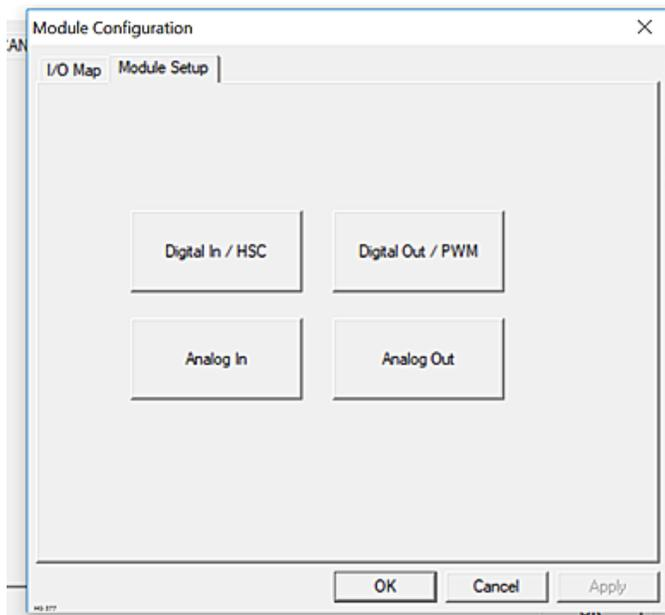
Select **Digital In/HSC** to open the Digital / HSC Input configuration dialog for a specific controller.
