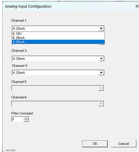
The Channel x drop down windows allow the user to specify the mode for each analog input to operate. The Channel x drop down windows are enabled/disabled according to which model is being configured. All of the models have the following modes available: 0..10V, 0..20mA, and 4..20mA.
