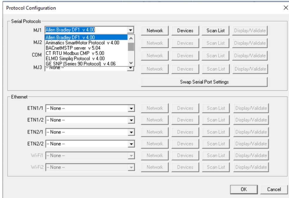
**NOTE:** If the MJ1 port is to be used in the Protocol Config, it will no longer be available for Cscape programming unless the controller is put into IDLE mode.
