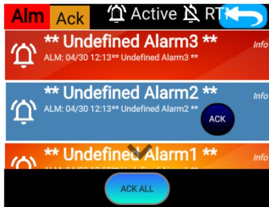
The currently selected entry is highlighted in blue color which can be moved up or down by directly touching an entry.
