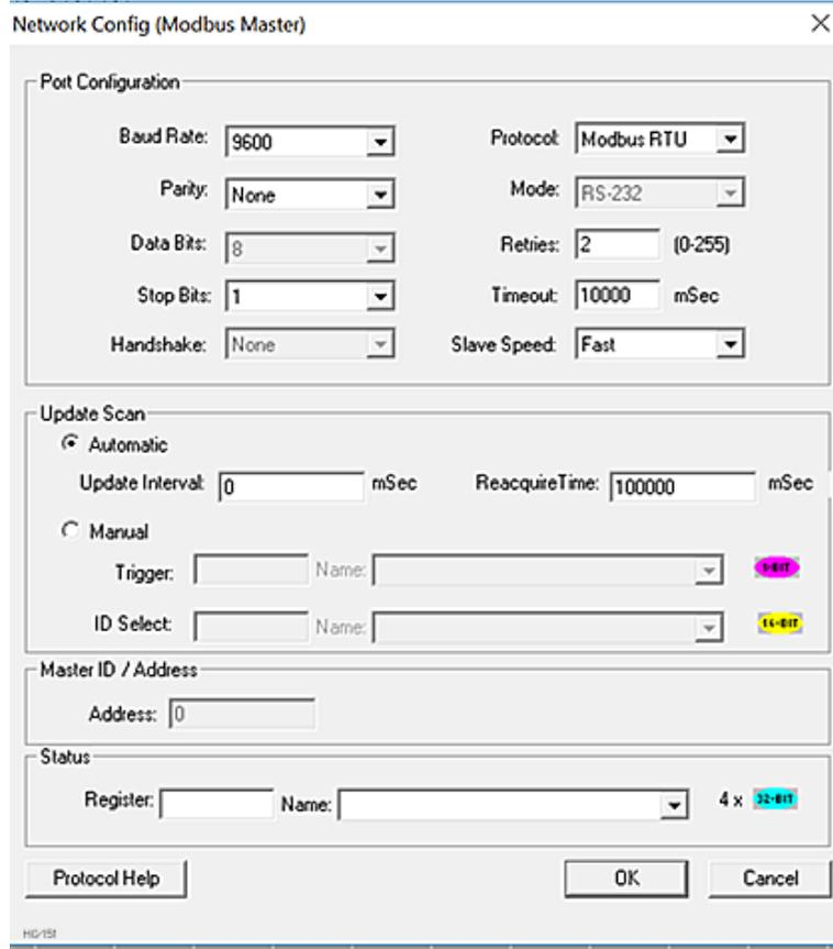
Network Configuration provides the required parameters to configure the network. Each protocol is different and may not require the entire Network Config field. Please refer to the table below for the options in the Network Config field.
