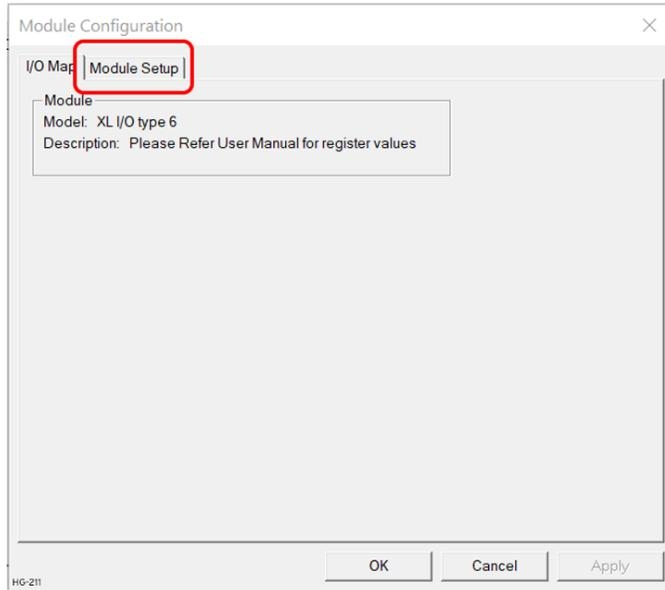
The Module Setup allows a user to configure four types of I/O. **NOTE:** Not all controllers offer all four types. Refer to the controller's datasheet on the using Horner's [Documentation Search](#) page.
