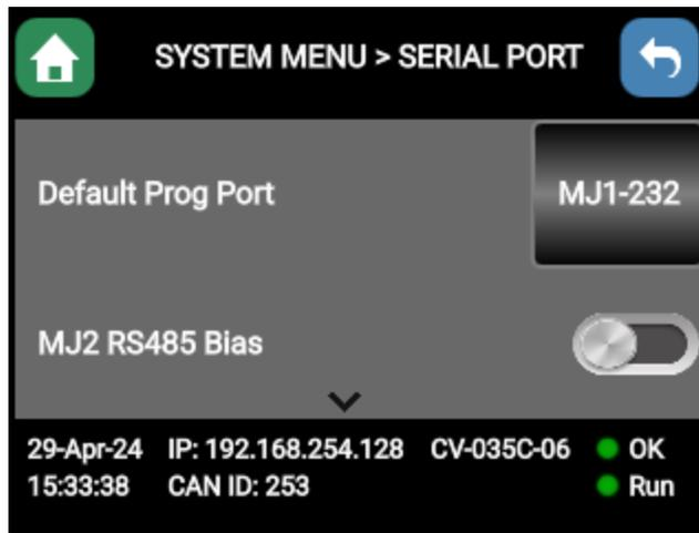
The Set Serial Ports Sub-Menu displays two System Settings, all of which are editable & displays three System Settings (View Protocol), none of which are editable.
