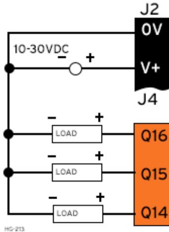
The digital outputs used in the OCS have electronic short circuit protection and current limiting. While these electronic protections work in most applications, some application may require external fusing on these outputs.
