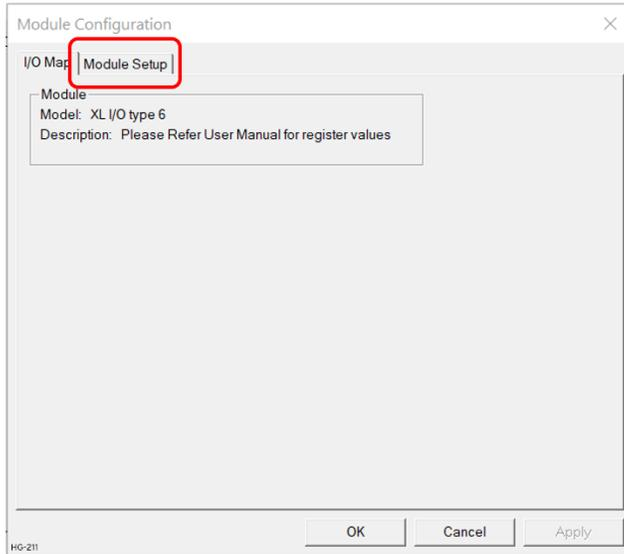
The Module Setup allows a user to configure four types of I/O. **NOTE:** Not all controllers offer all four types. Refer to the controller's datasheet the using Horner's [Documentation Search](#) page.
