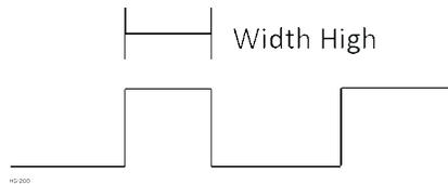
**Width Low 1  $\mu$ s Counts** – In this sub-mode the accumulator value will contain the number of 1  $\mu$ s counts the pulse is low.
