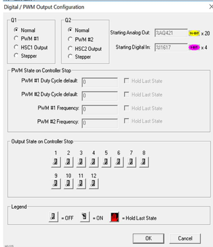
The **Q1** and **Q2** group boxes allow the user to specify the operation of the multifunction outputs.
