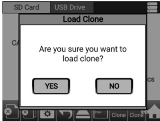
**Step 4:** After confirmation, all unit settings and register values will be loaded from Removable media to the Battery backed RAM (Regardless of AutoLoad settings) and then OCS resets for the settings to take effect.
