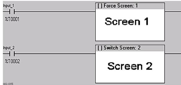
There is also a system register that can be used to for control-based screen navigation. %SR1 can be read to determine the current screen or written to change the current screen. Refer to the On-Line help in Cscape for more information on control-based screen navigation.
