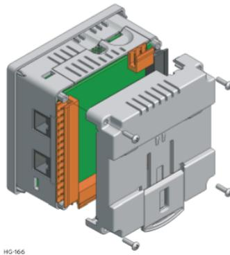
Once the back is removed the jumper selection can be changed. The jumper settings are documented on each data sheet using a diagram such as the figure below and a description of the jumper settings.
