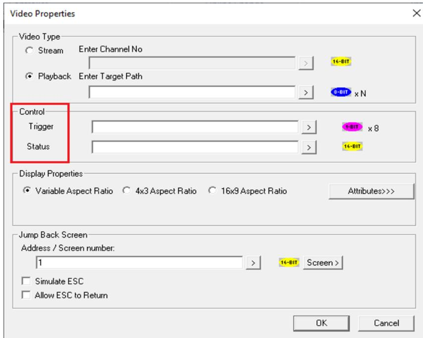
**Trigger** - The video control trigger is used to start, stop and pause video. Video trigger is done by bit level addressing. The trigger reserves eight (8) bits and uses the first two (2) bits.
