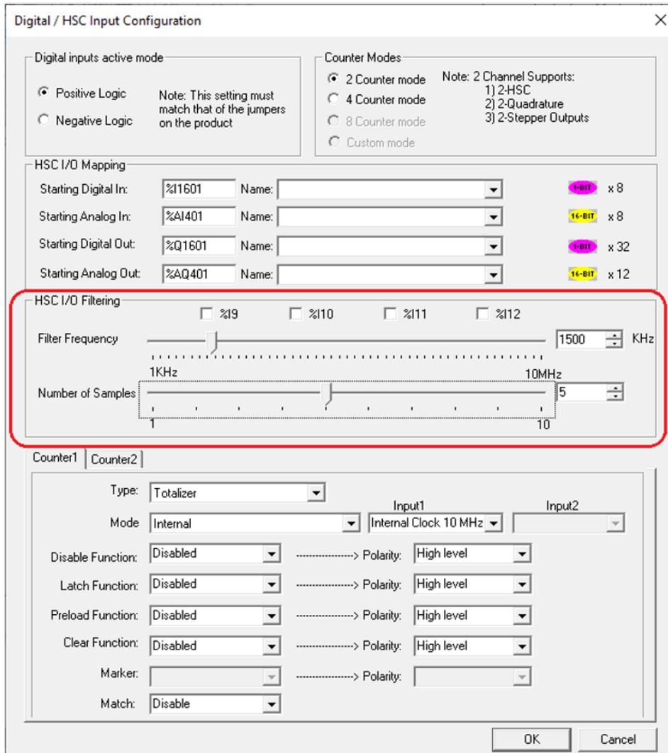
Input signal is filtered based on the filter frequency and Number of samples selected. User has to select Filter Frequency and Number of samples based on the frequency of the Input signal.
