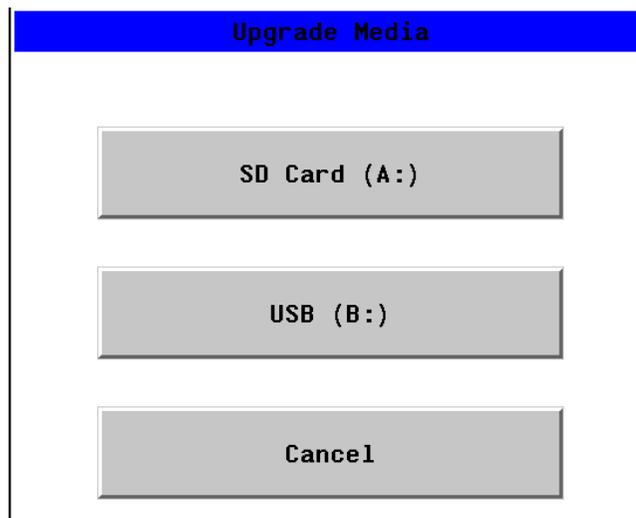
3. Select "SD Card (A:)" for upgrading firmware from microSD card or USB (B: ) for upgrading firmware from USB. Firmware upgrade will be started with appropriate message being displayed.
