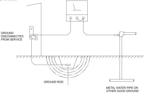
Figure 4.1 - Two-Point Ground Connection Test
