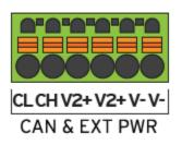
CAN communications are provided via three connectors on the CAN connector: CAN\_LOW (CL), CAN\_HIGH (CH), and V- (C).
