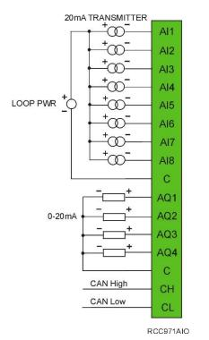
For CAN wiring, use the following wire type or equivalent: Belden 3084, 24 AWG (0.2mm<sup>2</sup>) or larger.
