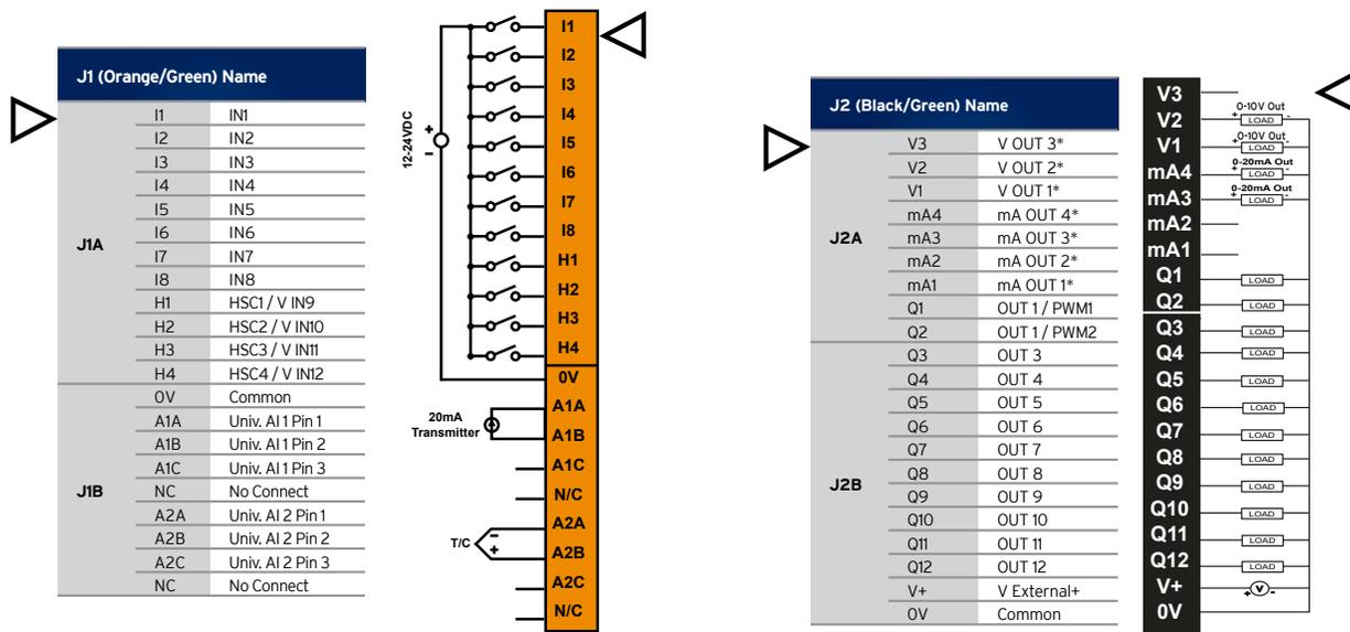
NOTE: \* Both mA & V outputs are active for each output channel, however, only the configured output type is calibrated (maximum 4 channels simultaneously).
