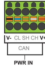
A single 5-pin connector is used to make both a network connection and power input. A quality Class 2 power supply should be used for this product. If the power is run with the network cable, care must be taken so that the voltage does not drop below the lower supply limit on longer runs.
