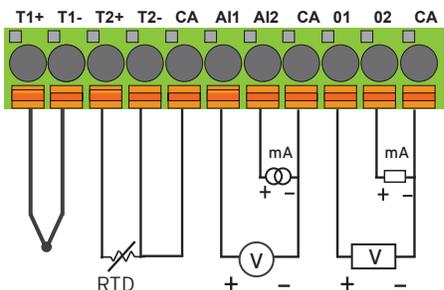
**J1:** CA terminals are internally connected together and isolated from BUS.
