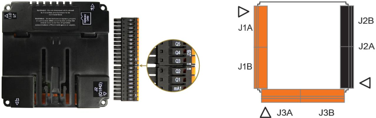
For ease of operability, the high density terminals are divided into more manageable pairs of connectors (J1A + J1B, J2A + J2B, J3A + J3B). To ensure proper installation, connector symbols must match.
